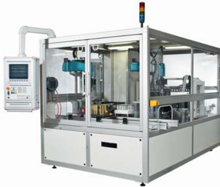
Cell to system: assembly of individual cells into battery systems (source: Manz Automation)
